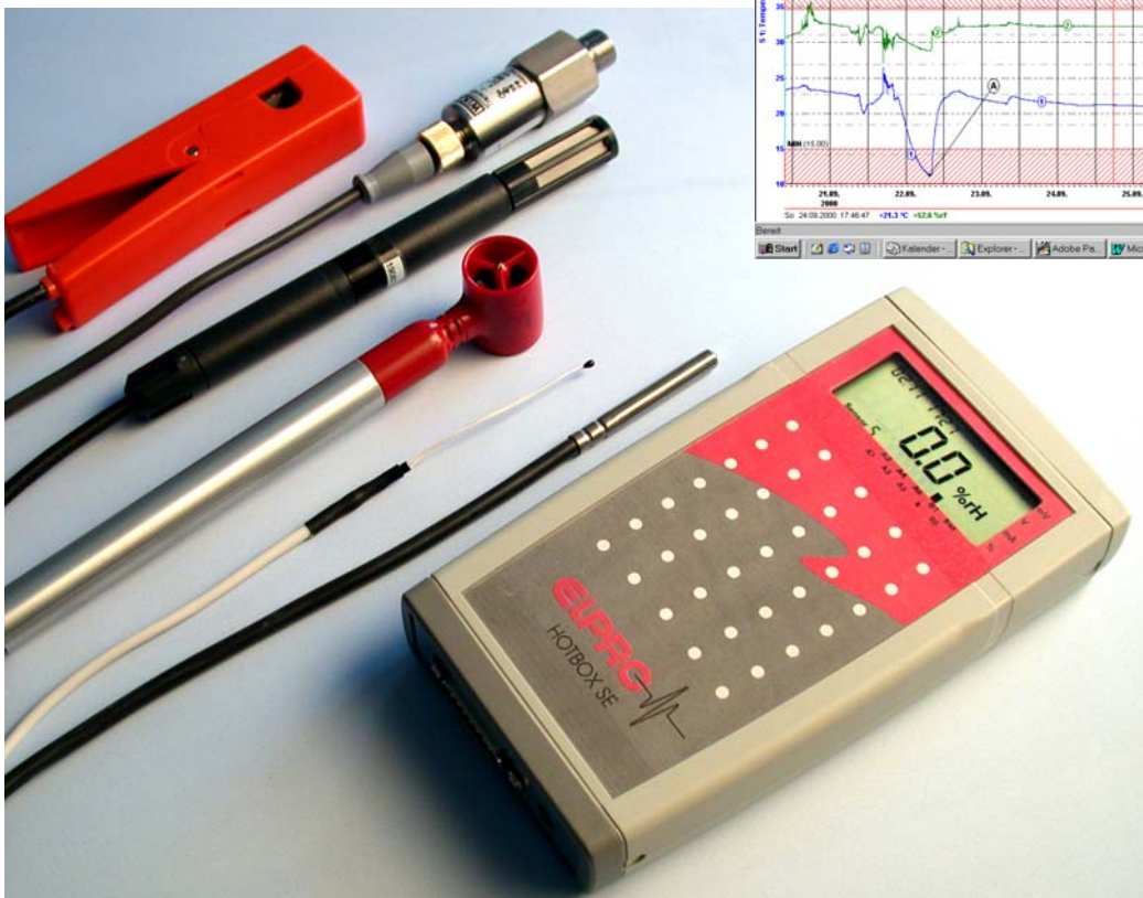
HOTBOX SE with different sensors
